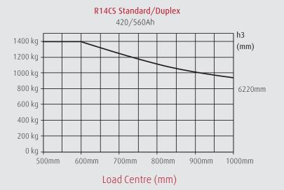
With STD 1010mm high load backrest, the mast max height will increase 430mm(STD fork carriage) or 535mm (Integrated side shift) Lift height = h3 + s + 15 mm
